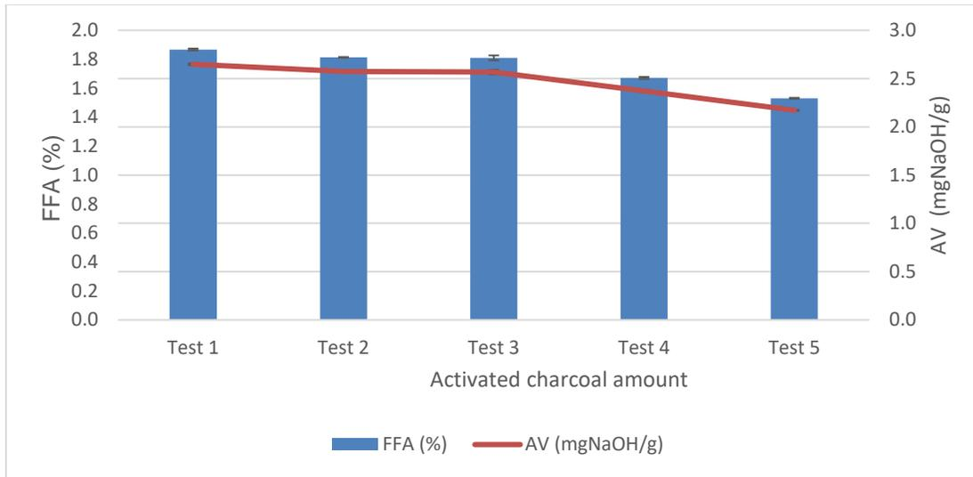
**Figure 1: Acid Value and Free Fatty acid value in absorbent deodorizing tests.**
