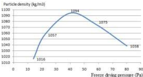
**Figure 2: Effect of freeze drying pressure (Pa) to particle density ( $\text{kg/m}^3$ ) of freeze-dried *Cordyceps militaris***
