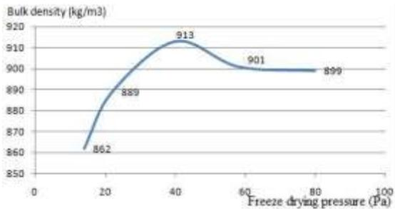
**Figure 1: Effect of freeze drying pressure (Pa) to bulk density ( $\text{kg/m}^3$ ) of freeze-dried *Cordyceps militaris***
