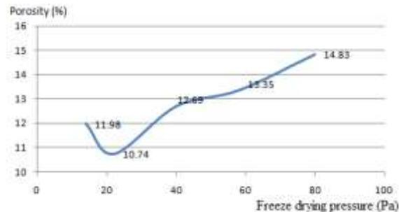
**Figure 3: Effect of freeze drying pressure (Pa) to porosity (%) of freeze-dried *Cordyceps militaris***
