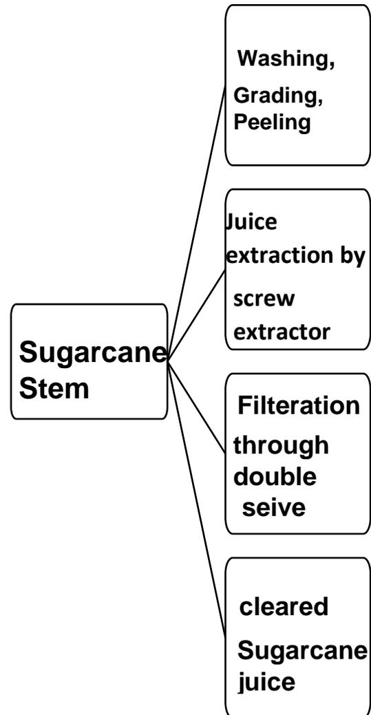
**Figure 1: Method for extraction of sugarcane Juice**
