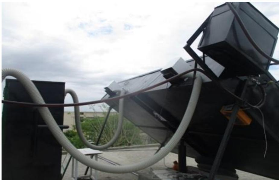
**Figure 2: The Flat Plate Solar Collector with drying chamber**
