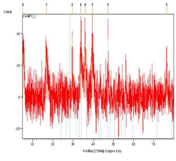
Figure 2: XRD analysis of Cu nanoparticles
