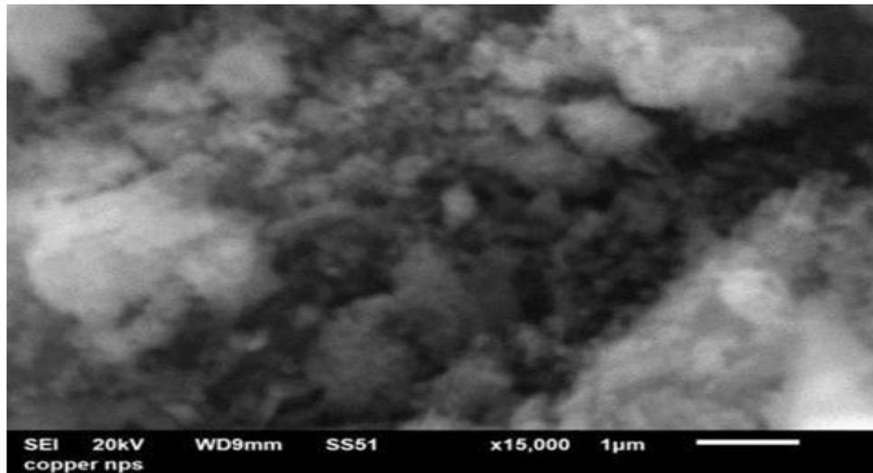
Figure 6: SEM images of Cu nanoparticles
