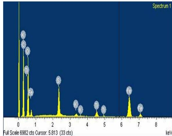
Figure 3: EDX of Fe nanoparticles
