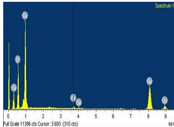
Figure 4: EDX of Cu nanoparticles
