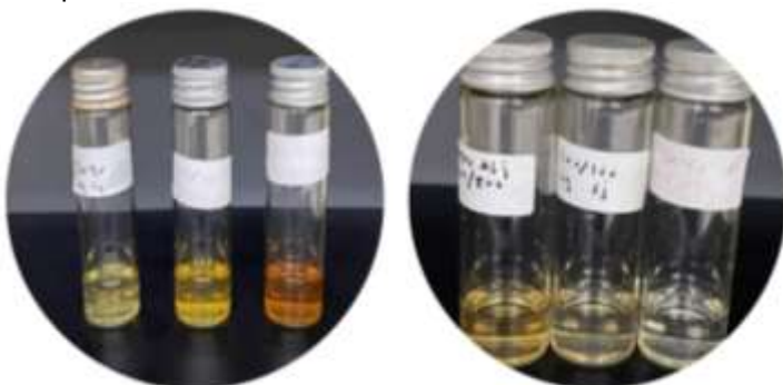
Figure 1: Preparation AgNPs; Colour change of leaf extracts before and after reduction by plant extract.
