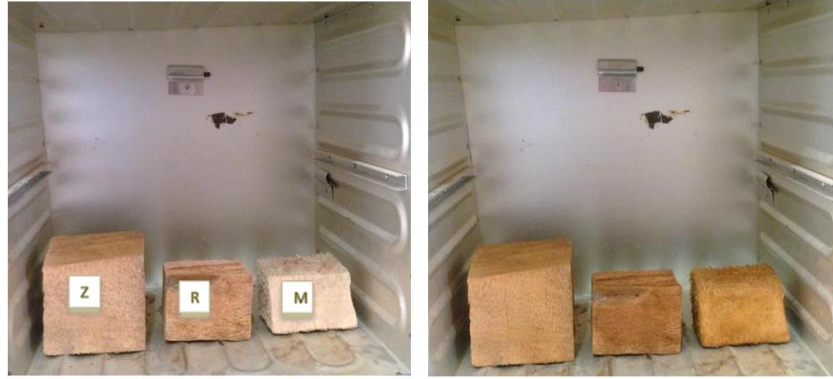
Figure 2. A) Primary specimens laid out in the oven (from right side it names Mazafati, Rabbi and Zardan); b) dried specimens after three days
