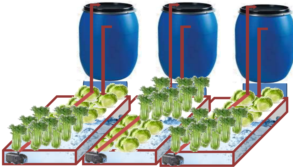
Figure 3: Air supply system deep flow technique (DFT) via submersible pump (40 watt) in deep water culture (DWC).
