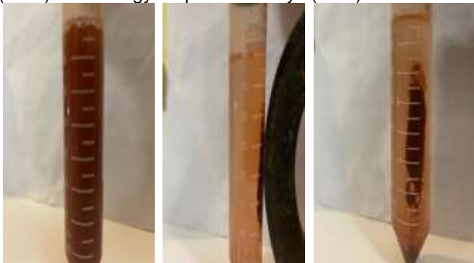
Figure 8: Attracted with magnet and without attracted MNPs.
